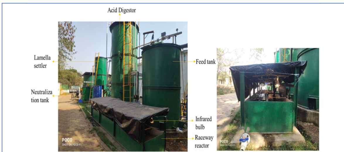
Overview of the implementation area 1.1 – Pilot scale anaerobic digester coupled with PHBR
