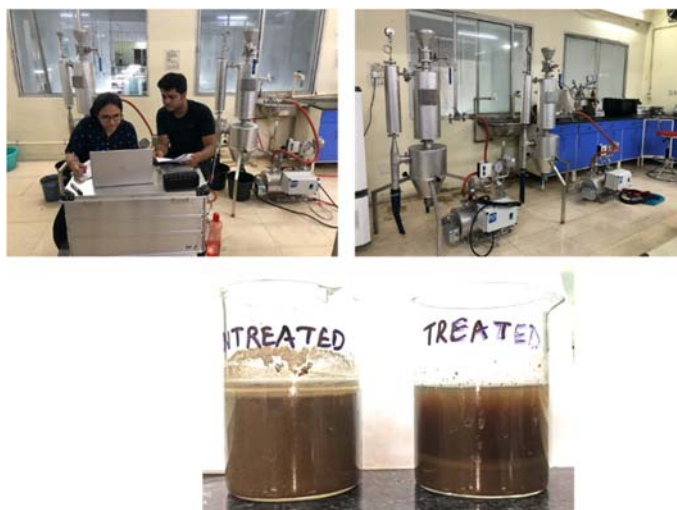
Picture – Commissioning of THP pilot. Top left: Commissioning with Cambi personell attending remotely. Top right: Pilot assempled and ready for commissioning. Bottom: Untreated sludge to the left, and treated sludge to the right.
