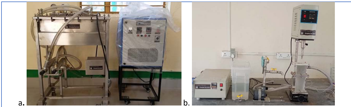
Overview of the implementation area 1.1 – a. Pilot scale sludge treatment system and b. Bench top ultrasound reactor
